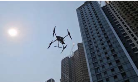
Drone-Based Exterior Wall Quality Improvement
